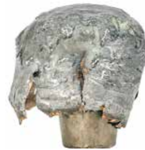
Prototype Terminal Ascent bullet upsets taken at a velocity of 2,757 feet-per-second.
