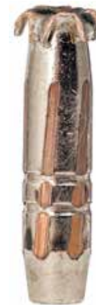
Prototype Terminal Ascent bullet upsets taken at a velocity of 1,350 feet-per-second.
